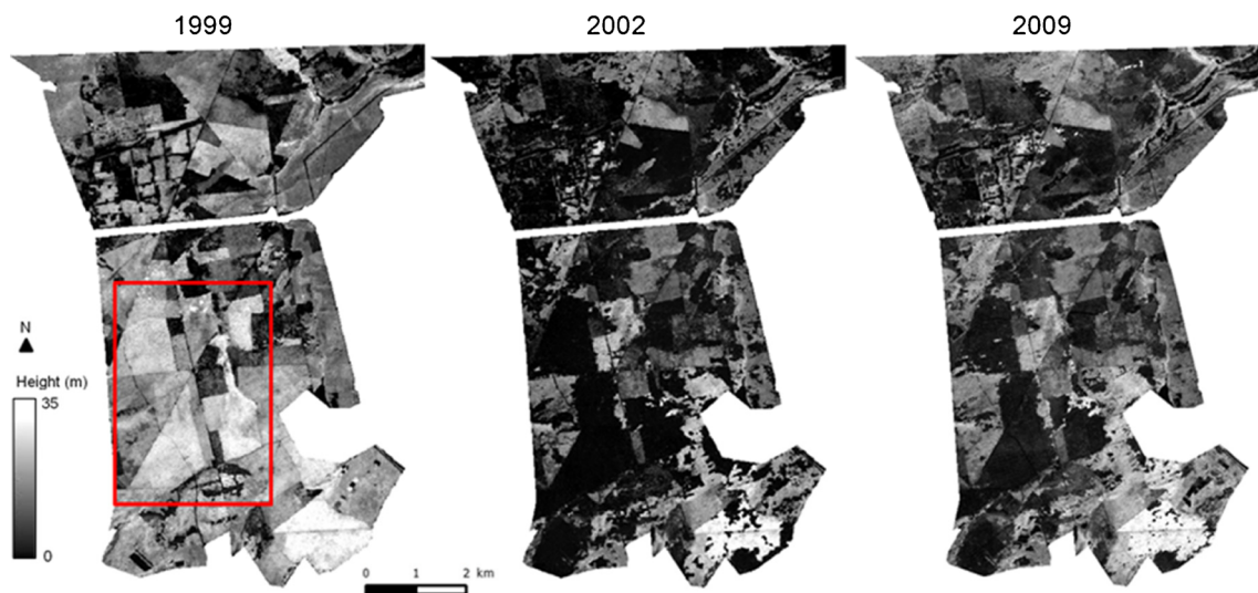
Fig. 1 Illustration of photogrammetric canopy height models for 1999, 2002, and 2009. Gray levels (from dark to white) represent increasing height in meters. In 1999, the area of interest is presented as a red rectangle
