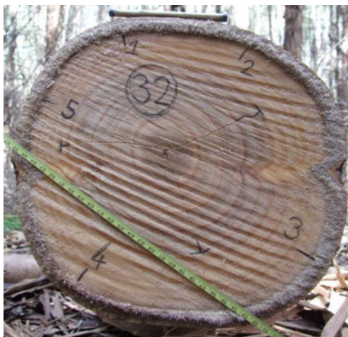
Fig. 2 Example of a butt log cross-section picture showing strain gauge locations (numbered 1–5), and cracks in the centre of the log observed few minutes after felling the tree
