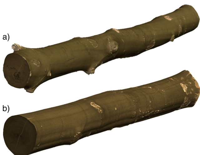
Fig. 1 3D reconstructions of computed tomography (CT) images of two example logs: a crooked log of quality grade “D” (log “B3”) and b higher-quality log of grade “B” (log “D1”)
