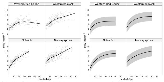
Fig. 1 MOE plotted by ring number from the pith. Left, observed values. Different sites are represented with different plotting symbols (+= north latitude,  $\Delta =$  middle latitude, O = south latitude) and locally weighted regressions are plotted as trendlines. Right, marginal predictions from the model
