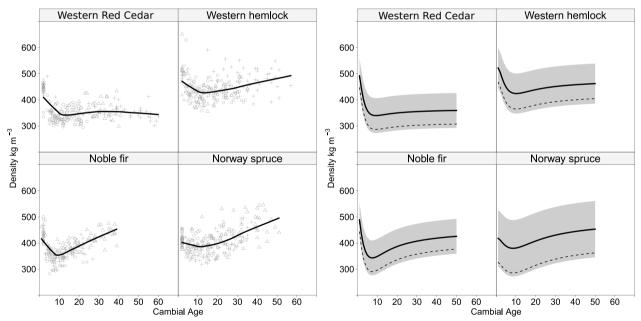
Fig. 3 Wood density plotted by ring number from the pith. Left, observed values. Different sites are represented with different plotting symbols (+=north latitude,  $\Delta$ =middle latitude, O=south latitude) and locally weighted regressions are plotted as trendlines. Right, marginal predictions from the model
