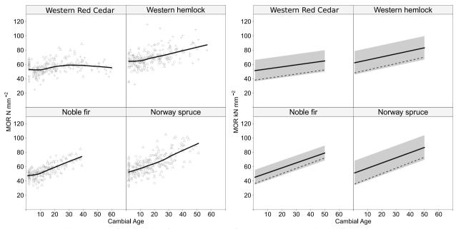
**Fig. 2** MOR plotted by ring number from the pith. Left, observed values. Different sites are represented with different plotting symbols  $(+= north | atitude, \Delta = middle | atitude, O = south | atitude)$  and locally weighted regressions are plotted as trendlines. Right, marginal predictions from the model
